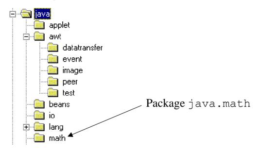
The root of any package must be accessible through a Java system default directory or through the CLASSPATH environment variable
